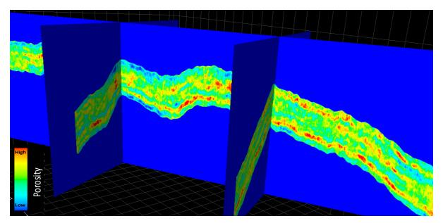
Figure2 Porosity volume after seismic inversion.
