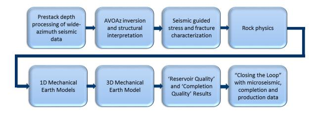
*Figure 1* Workflow used to determine in-situ stress, stress anisotropy, geomechanical properties, and the density and orientation of natural fractures in unconventional reservoirs.
