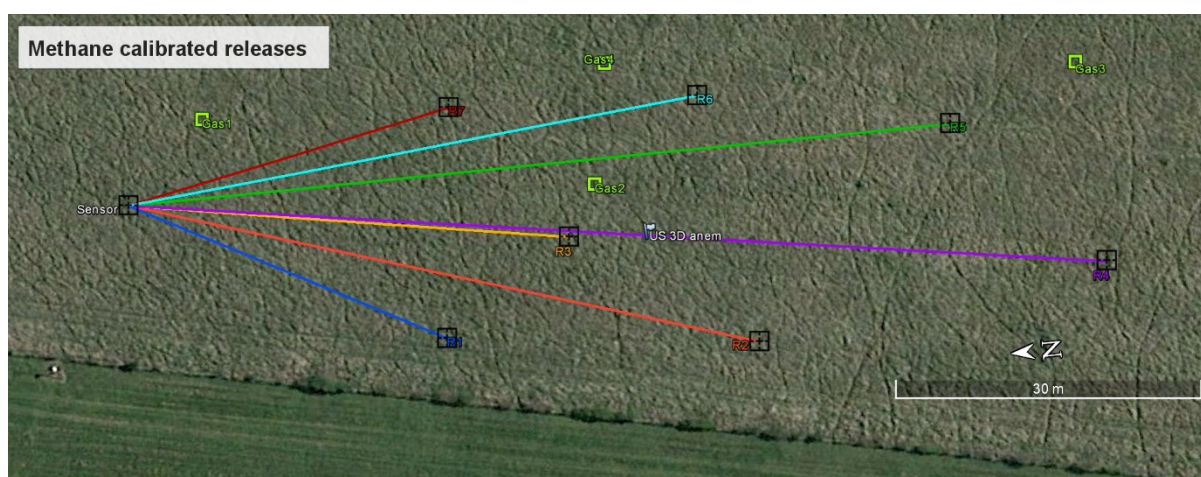
Figure 1 Top view of the spatial arrangement of the sensor, retroreflectors, gas release locations and ultrasonic 3-D anemometer at the Chilbolton Observatory Hampshire, UK. The green squares indicate gas release locations, the black boxes the retroreflector locations and the grey flag the weather station location.
