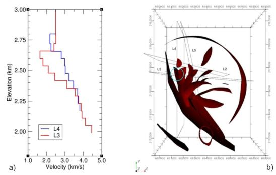
*Figure 3* a) Comparison of P-velocity profiles at the cross between sub-perpendicular L4 and L3 evidences different velocities with possible anisotropy. This zone is characterized by the presence of a shallow fault as shown by the small blue circle in (b) (modified after Calcagno et al., 2018).
