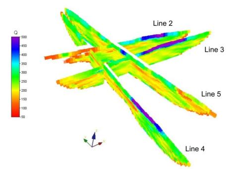
Figure 2 3D view of the tomographic inversion for attenuation of the Los Humeros seismic lines.
