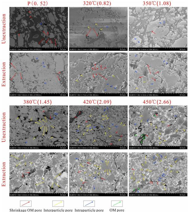
**Figure 1** The SEM images showing the evolution characteristics of pores in shale rocks from the pyrolysis experiments in this work (data in the parentheses showed the values of  $EasyR_o$ ).
